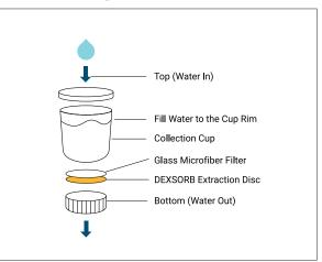
Powered by DEXSORB®: WTK uses our DEXSORB® adsorbent to extract PFAS at the point of testing, preserving the sample in its on-site condition and eliminating the need to ship water to a lab. Easy, Accurate, Affordable!
