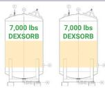
DEXSORB packed bed filtration (two 7,000-lb vessels) for removal of PFOS and 6:2 FTS; Replace 7,000 lbs DEXSORB every 36 weeks
